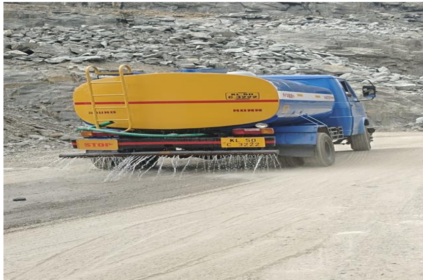
Figure:6 Photographs showing water spraying on quarry road for dust suppression.
